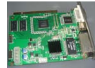
Main control card (Installed PC)
